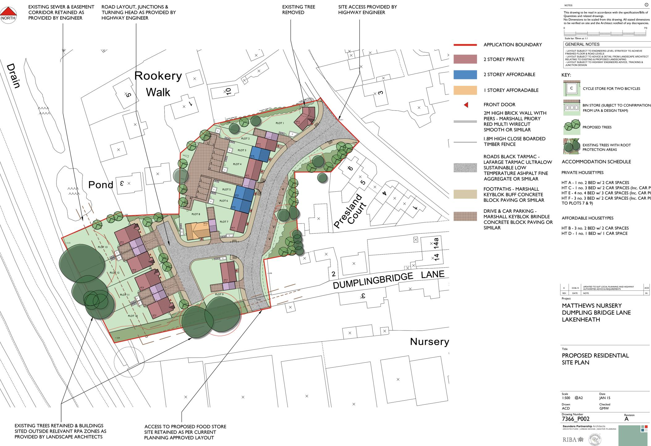
to be verified on site and the Architect notified of any discrepancies.
